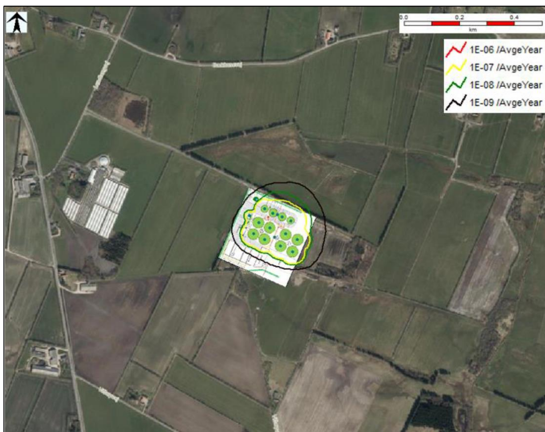
Figur 14.3 - ISO-risikokurver for Outrup Biogas ApS.
